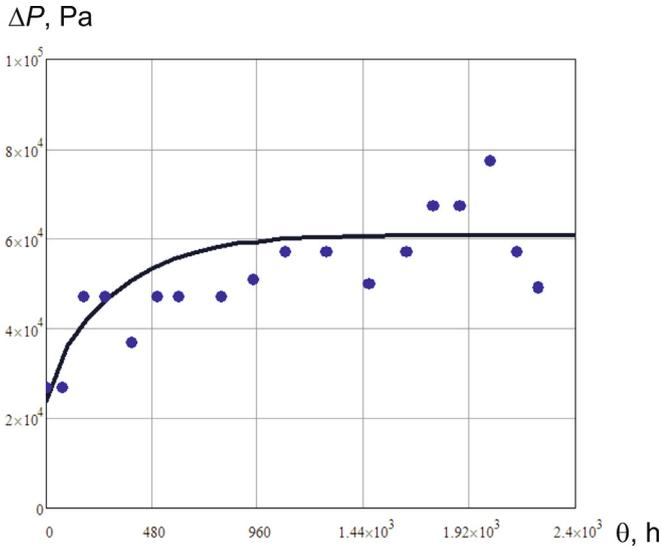
Fig. 3. Pressure loss in PHE for thin sugar juice heating of Case study 1: solid curve is calculated; dots are test results.
