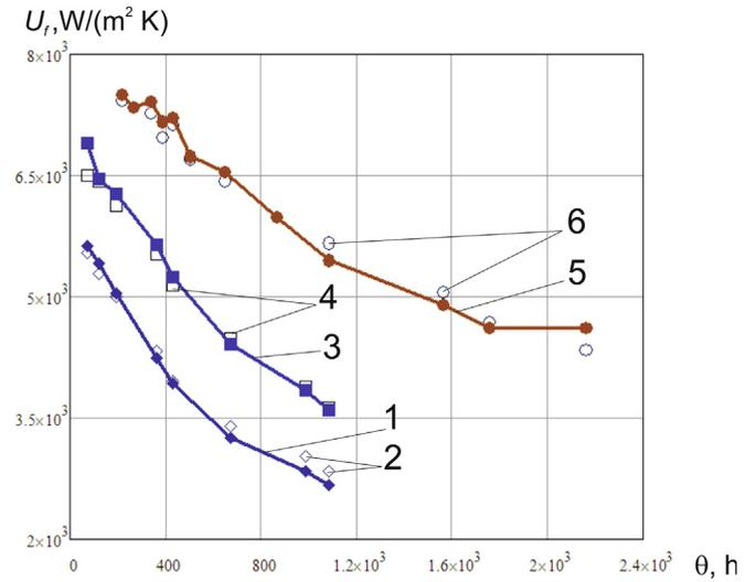
Fig. 4. Tests data (empty dots) and calculated by model results (solid dots) for overall heat transfer coefficients in PHE of Case study 2 at different flow velocities: 1,2 – 0.26 m/s; 3,4 – 0.4 m/s; 5,6 – 0.57 m/s.
