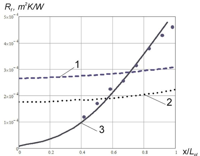
Fig. 2. Calculated local thermal resistance of fouling in PHE channel. Case study 1: (1) –28 d of operation; (2) –13 d of operation. Case study 2: (3) –28 d of work at flow velocity  $w_2 = 0.26$  m/s; experimental values are shown by dots.
