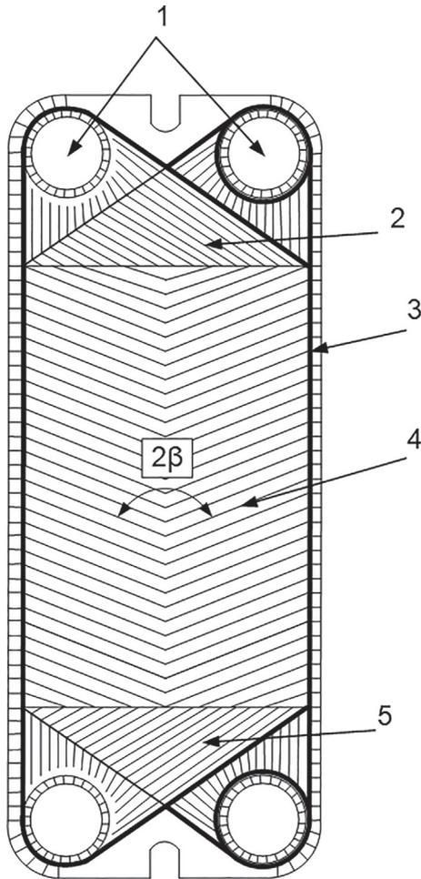
Fig. 1. Sketch of PHE plate area: 1 inlet and outlet of streams; 2, 5 flow distribution zones; 3 elastomeric gasket; 4 the main area of the corrugated field.
